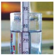
3. The alcohol meter shown in this information pamphlet is for use with ethanol; if used to control an isopropanol solution, a 75% solution will show 77% (± 1%) on the scale at 25°C.
