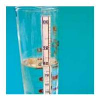
2. Post-production analysis is mandatory if either ethanol or an isopropanol solution is used. Use the alcohol meter to control the alcohol concentration of the final use solution. The accepted limits should be fixed to  $\pm$  5% of the target concentration (75%–85% for ethanol).
