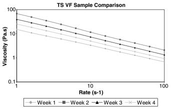
**Figure 3.6c** Viscosity profile of thickshake videofluoroscopy fluid sample over weeks 1 to 4. Graph shows viscosity (Pa.s) versus rate  $(s^{-1})$
