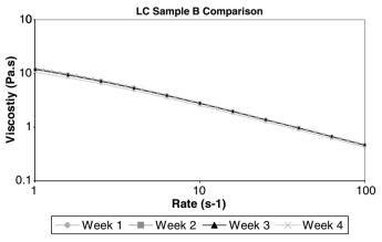
**Figure 3.5b** Viscosity profile of lemon cordial dietary B fluid over weeks 1 to 4. Graph shows viscosity (Pa.s) versus rate  $(s^{-1})$
