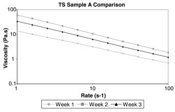
**Figure 3.6a** Viscosity profile of thickshake dietary fluid sample A over weeks 1 to 3. Graph shows viscosity (Pa.s) versus rate  $(s^{-1})$
