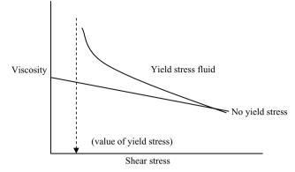
Figure 3.2 Yield stress determination of fluids from viscosity-shear stress data
