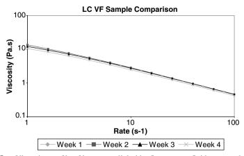
**Figure 3.5c** Viscosity profile of lemon cordial videofluoroscopy fluid over weeks 1 to 4. Graph shows viscosity (Pa.s) versus rate  $(s^{-1})$
