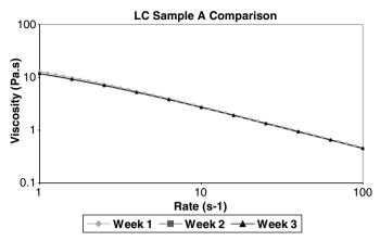
**Figure 3.5a** Viscosity profile of lemon cordial dietary A fluid over weeks 1 to 3. Graph shows viscosity (Pa.s) versus rate  $(s^{-1})$
