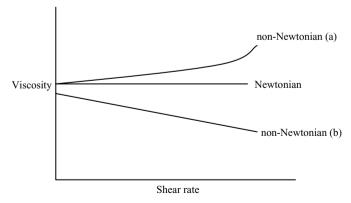
**Figure 3.3** Viscosity profiles of Newtonian and non-Newtonian fluids (a) shear thickening, (b) shear thinning
