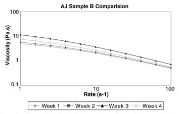
**Figure 3.4b** Viscosity profile of apple juice sample B dietary fluid over weeks 1 to 4. Graph shows viscosity (Pa.s) versus rate  $(s^{-1})$
