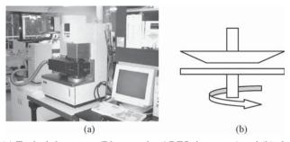
Figure 3.1 (a) Typical rheometer (Rheometrics ARES rheometer) and (b) close-up sketch of cone and plate fixture used in rheometer
