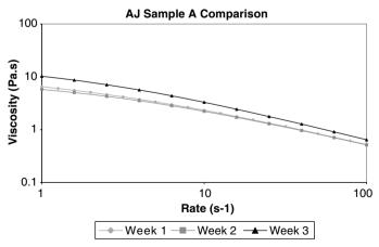
**Figure 3.4a** Viscosity profile of sample apple juice A dietary fluid – comparison over weeks 1 to 3. Graph shows viscosity (Pa.s) versus rate  $(s^{-1})$
