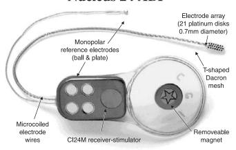
Figure 2. Implantable portion of the ABI, showing the receiver/stimulator and electrode array.
