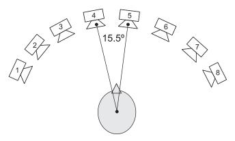
Figure 3. Eight-speaker localization test set-up. Speakers are at 15.5.° (From Van Hoesel and Clark, 1999.)
