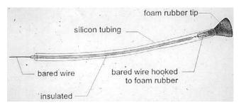
Figure 2. Construction of a tympanic membrane electrode (foam rubber tip can be replaced with soft cotton). (From Ferraro, 2000, p. 434.)
