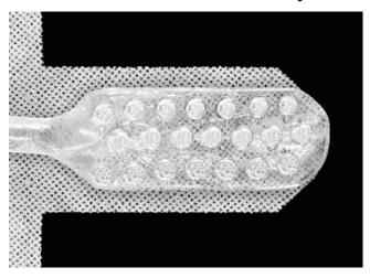
**Figure 3.** Close-up view of the 21-electrode array, which consists of 21 platinum disks mounted on a Silastic substrate. The fabric mesh backing is intended to encourage fibrous ingrowth to fix the electrode array in position.
