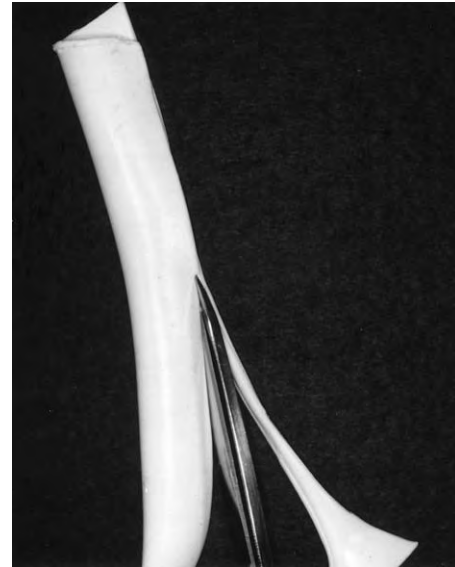
Fig. 9-8 Simultaneous cutting of bonded pieces creates a smooth single edge.
