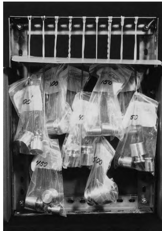
Fig. 7-8 Standard brass weights were attached to no. 33 high-quality rubber bands and suspended from the tension adjustment frames.
