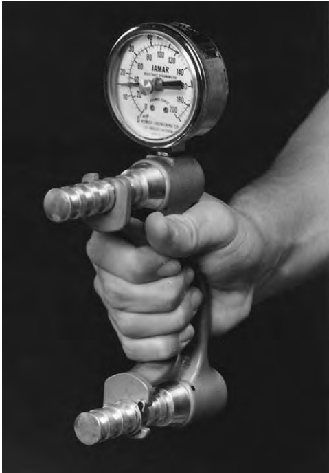
Fig. 5-13 Maximum grip strength depends on the size of the object being grasped. Normal values for the five handle positions form a bell-shaped curve.
