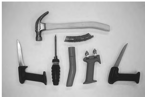
Fig. 17-9 Shock-absorbing material applied to tools, equipment, or instruments decreases pressure on an irritated A-1 pulley.
