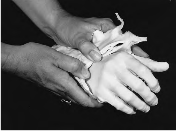
Fig. 24-17 Because the materials are heterogeneous, the silicone rubber negative mold is easily peeled from the positive without the need for an intervening separator substance.
