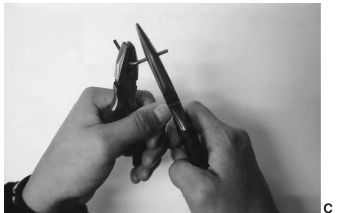
Fig. 9-10 A, Applying force at a point distal to the intended bend provides a longer lever arm with which to shape wire. B,C, Different types of pliers ease bending wire to specific angles or curves.
