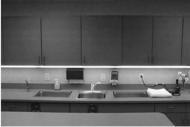
Fig. A-3 A counter insert for a hot water pan is strategically placed close to the splint fabrication worktable, providing an efficient workspace where water is maintained at a constant temperature appropriate for low-temperature splinting materials. The expanded size of the inserted pan allows immersion of larger pieces of materials or splints and a valve situated beneath the pan facilitates drainage. Positioned adjacent to the insert pan, a faucet simplifies quick cooling of heated materials and filling of the pan. On the opposite side of the pan, a heat gun and a towel for cooling and drying materials prior to fitting are situated.
