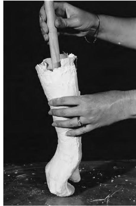
Fig. 24-14 A dowel rod or similar object incorporated into the positive mold at the time of pouring allows the finished mold to be secured in a vise, display stand, etc.
