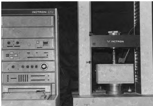
Fig. 6-41 The experimental setup showing the Instron testing machine with the foam test specimen in place.
