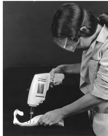
Fig. 9-4 Safety precautions should be carefully observed when working with hand tools or power equipment. A , Incorrect. B , Correct.
