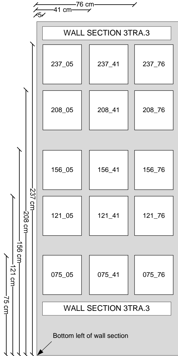
Figure 15 – Example of non-vertically aligned patch panel identification
