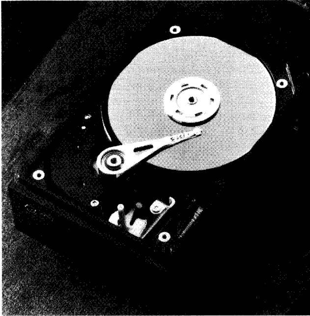
FIGURE 4-6. Hard-disk drive. A read/write head is visible at the end of the arm overlying the top disk platter. (Photograph courtesy of Seagate Technology, Inc.)
