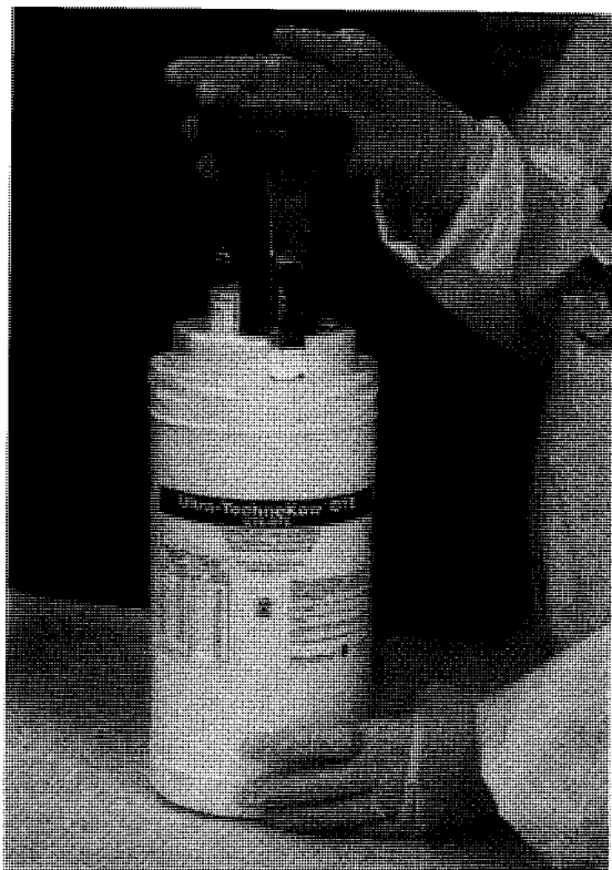
FIGURE 19-7. Picture of a "wet" molybdenum 99/technetium 99m generator and cross-sectional diagram of the generator. (Adapted with permission of Mallinckrodt Medical Inc., St. Louis, MO.)
