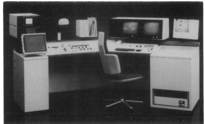
Figure 17.5(b) Gamma camera control console. Note that a computer display screen on the right hand side enables digitised information from the gamma camera to be displayed. The oscilloscope on the left has a persistent image for operator viewing and below it a 10"×8" compact recording camera produces permanent copies for a second, rapid fade oscilloscope.
