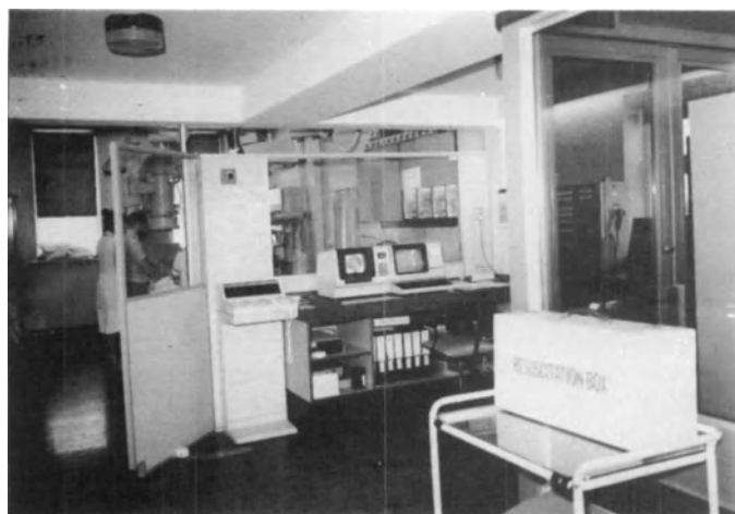
Figure 20.2 Control area. Fluoricon 3000 digital system housed in air conditioned cabinet in right foreground
