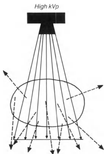
Figure 7.2 High kVp. A greater proportion of the radiation is scattered in a forward direction, thus more scatter reaches the film
